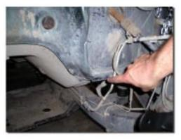
around the engine heads and above both of the exhaust manifolds). Mark these spots with a pen, remove engine, and clearance the firewall accordingly. Lower the engine back in and check the
