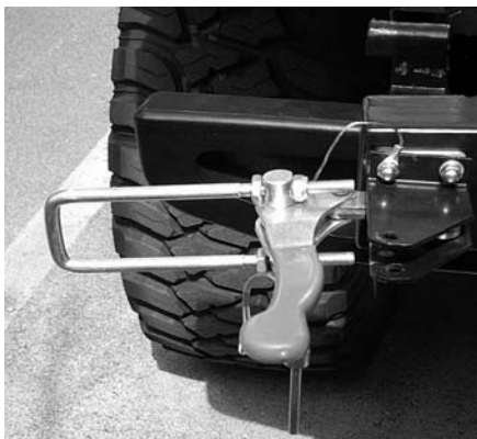
Photo 3 - Latch and latch-plate. Adjust latching "U-bolt" so it takes no more than 25lbs to latch handle and remain closed. More than this amount of torque to latch could result in damage to the "U-bolt" and / or latch-plate and bolts over time.
