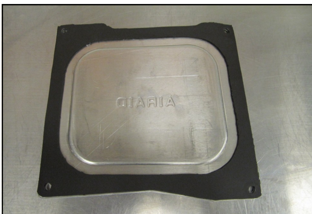
19. Place the Gasket (#8) onto the underside of the Air Box Lid (#4) and peel off the protective film. Mount the lid on the Air Box using four 1/4-20 x 1/2" Button Head Bolts (#18), and 1/4" Flat washers (#11).
