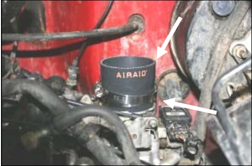
17. Install the reducer (#6) onto the throttle body using two #44 hose clamps (#16). Tighten only the hose clamp on the throttle body for now..
