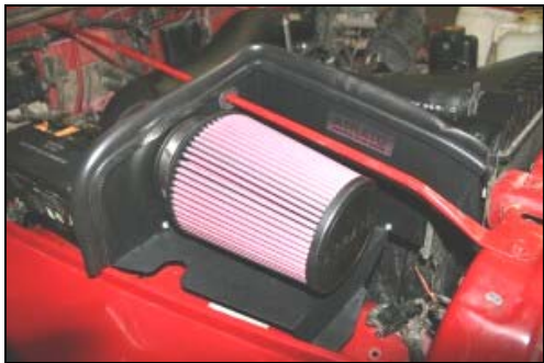
22. Install the Airaid Premium Filter (#1) onto the CAD tube and tighten the hose clamp. Next, install the weather strip (#7) onto the top of the CAD as shown, starting at the fender, working your way towards the radiator.
