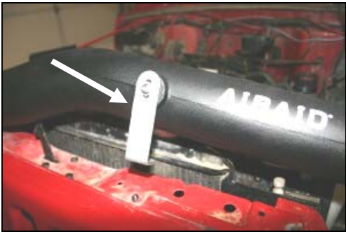
18. Install the L-bracket (#18), onto the Airaid Intake Tube (#4), using one 1/4" button head bolt (#11), and flat washer (#12). Leave the bolt loose for now.
