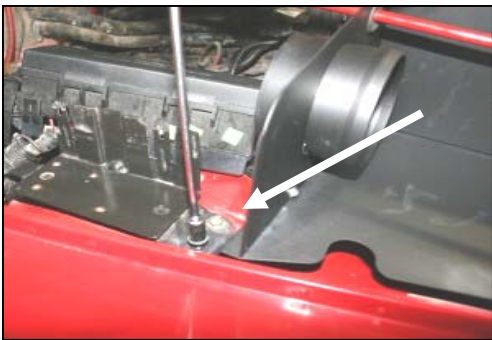
14. Re-install the factory bolt from step # 8 thru the CAD , and into the fender. Re-install the fuse box on the factory mount.
