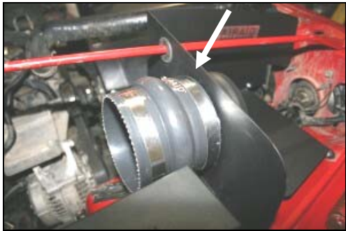
16. Install the urethane hump hose (#5) onto the back side of the CAD tube using two #72 hose clamps (#17). Tighten only the hose clamp on the metal tube for now.
