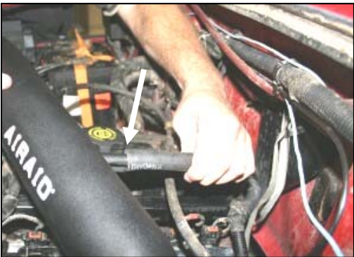
21. Re-connect the breather hose to the Airaid Intake Tube.
