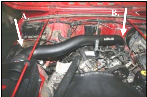
19. A.) Install the large end of the Airaid Intake Tube into the hump hose. B.) Now slide the small end into the reducer on the throttle body.
