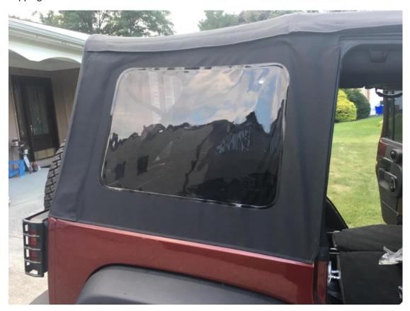
19. Zip the rear window up and slide the tailgate bar into the bottom of the window.
