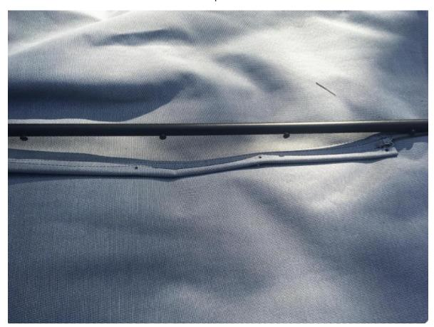
4. Remove the four screws in the back of the soft top frame.
