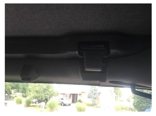
16. Pull down the rear of the soft top and push the plastic piece into the body rail.
