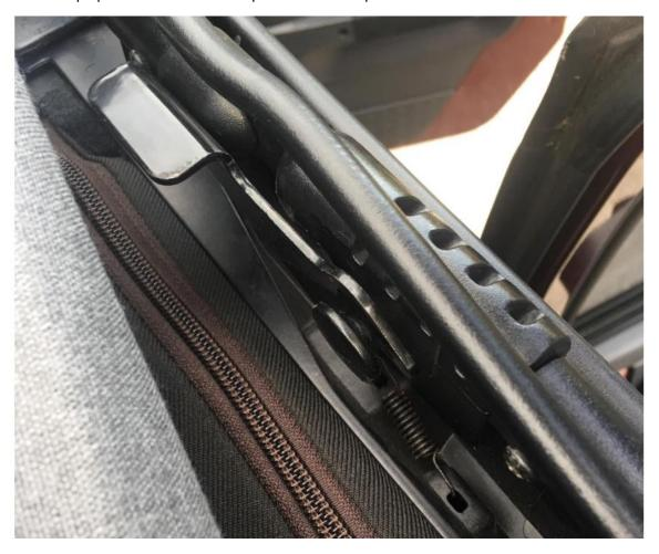
15. Flip the soft top over the driver and passenger seat and clip the two header clip to the window frame.
