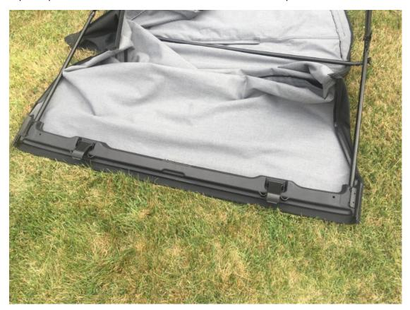
11. Reattach the four screws in the rear of the soft top to the frame.
