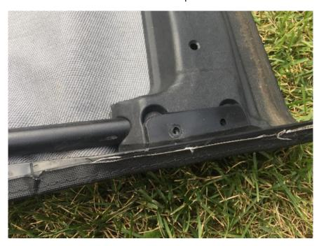
3. Remove the four screws in the middle of the soft top frame.
