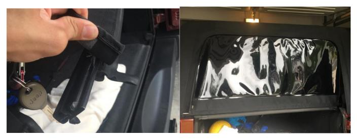
20. Attach the end of the tailgate bar into the brackets on each end of the tailgate.
