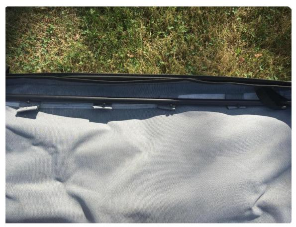
5. Flip the soft top forward to expose the header screws.
