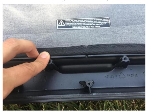
9. Tape the soft top to the soft top frame as shown.
