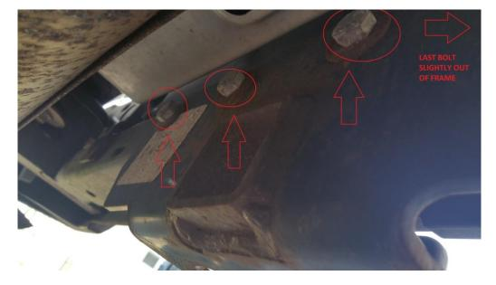
b. Use your open wrench to hold the lock nuts in place, as you loosen the bolts from the inside part of the frame as shown above
