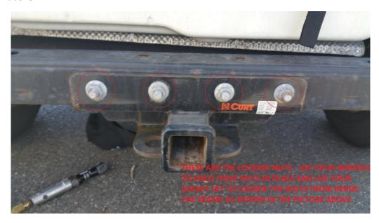
c. Once all four bolts are removed, simply pull the receiver hitch assembly straight down to remove it from the frame
