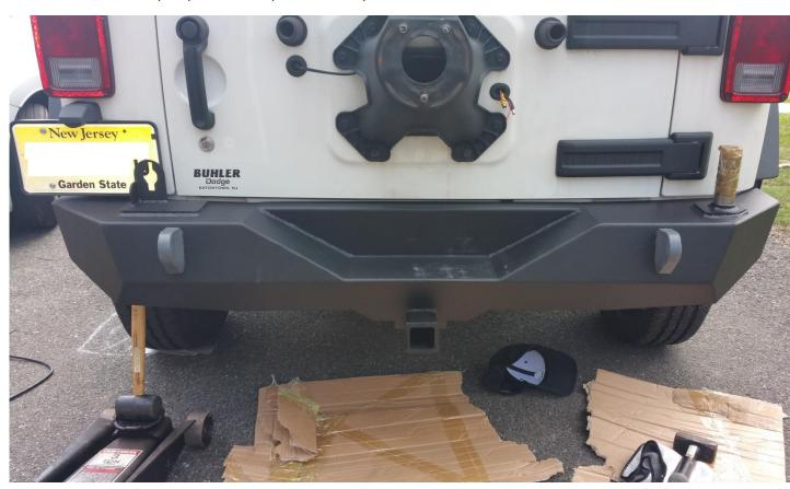
7. Using your 13mm socket or wrench, remove the 8 bolts holding on your stock tire carrier. Be sure to disconnect your 3<sup>rd</sup> brake light wire. If you don't want to damage the wire, you can use a T20 Torx bit to unscrew the back of the stalk, and unplug the wire)
