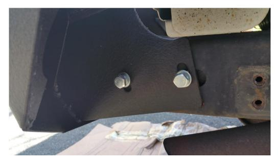
c. Underneath the frame, where the old receiver was (or wasn't), you have 4 empty bolt holes. You also have a 4 bolt hole reinforcing plate. This plate will be positioned as such:
