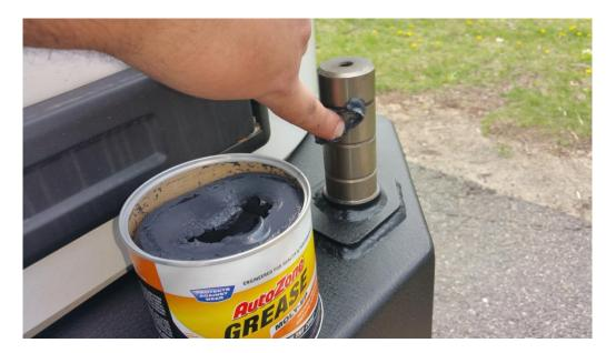
9. Place the tire carrier hinge cap on top of the hinge post, and secure tightly using the provided allen key screw (feel free to smear some grease on the threads of the screw to help keep moisture out of the hinge assembly)
