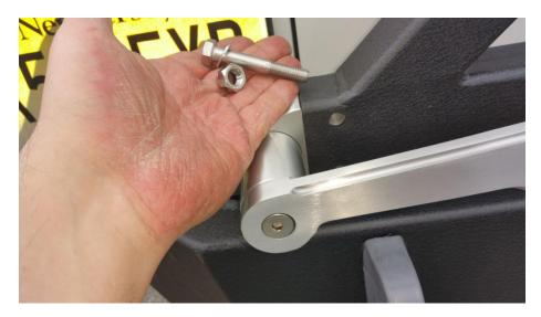
11. Secure the spare tire bracket to the tire carrier using the supplied 19mm hardware. Mounting height is subjective, based on how tall your tire is. I have a 29" tire and I've mounted on the lowest set of holes. Please note that the horizontal bolts can be loosened and the tire bracket can slide in and out to decrease or increase the space between the tire, and carrier.
