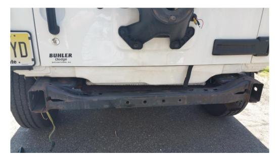
a. Identify the two bolt holes at the end of the frame rails (driver and passenger side) that you will use to mount the new Barricade bumper
