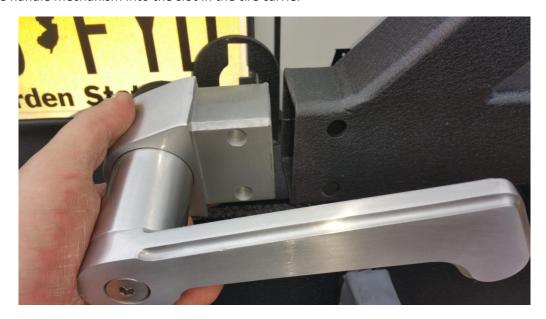
b. And secure using the provided 19mm bolts. The bolt gets one washer, is threaded through, and gets a locknut on the back.
