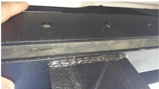
d. Using the long 19mm bolts, we will bolt through the reinforcing plate and frame. The long bolts will have a flat washer first, then thread the bolt through the plate and frame. On the back side of the bolt, add a flat washer and then the capture nut.
