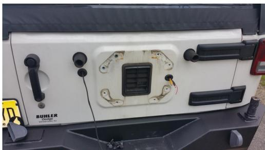
(the black wire hanging down is the brake light wire. You can remove the rubber grommet, stuff the wire into the tailgate, and get the grommet 95% back in to protect everything)
