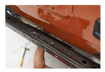
**STEP 4** // Install the mounting bracket to the inner side of the rear bumper support beam, slide the bolts through, leaving the nuts off.
