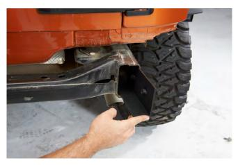
**STEP 5** // Next, slide the L-Shaped mounting brackets into the frame rails with the nut backing up to the predrilled hole in the frame.
