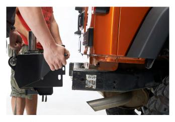
**STEP 6 //** Slide your new rear bumper over the brackets and bolts set in place in the previous steps.
