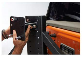
**STEP 13** // Finally, install the rear tire carrier and secure it to the rear swing arm at the desired height using the supplied hardware.
