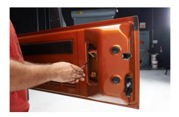
**STEP 2** // Disconnect the third brake light harness, which can be access through the rear panel of the tailgate.
