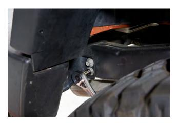
**STEP 3** // Remove the (4) 15mm bolts securing the rear bumper.
