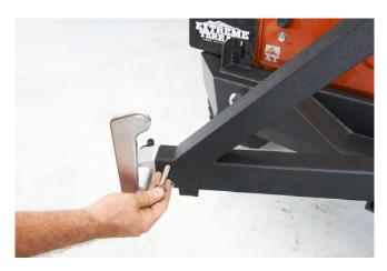
**STEP 11 //** Slide the latch into the end of the swing arm and secure with the two bolts and nuts.
