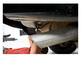
**STEP 8** // Using the supplied nuts, install the center support and tighten.
