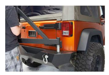
**STEP 9 //** Install the swing arm by sliding it over the post on the bumper. \*Note it may help to grease the post for smoother operation.
