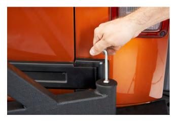
**STEP 10 //** Install the top cap then secure it with the supplied allen-head bolt.
