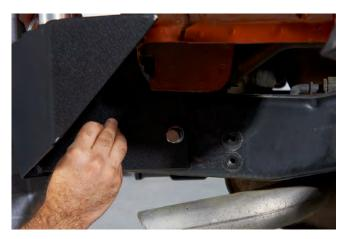
**STEP 7** // Thread the (4) supplied bolts into the side bumper supports and tighten.
