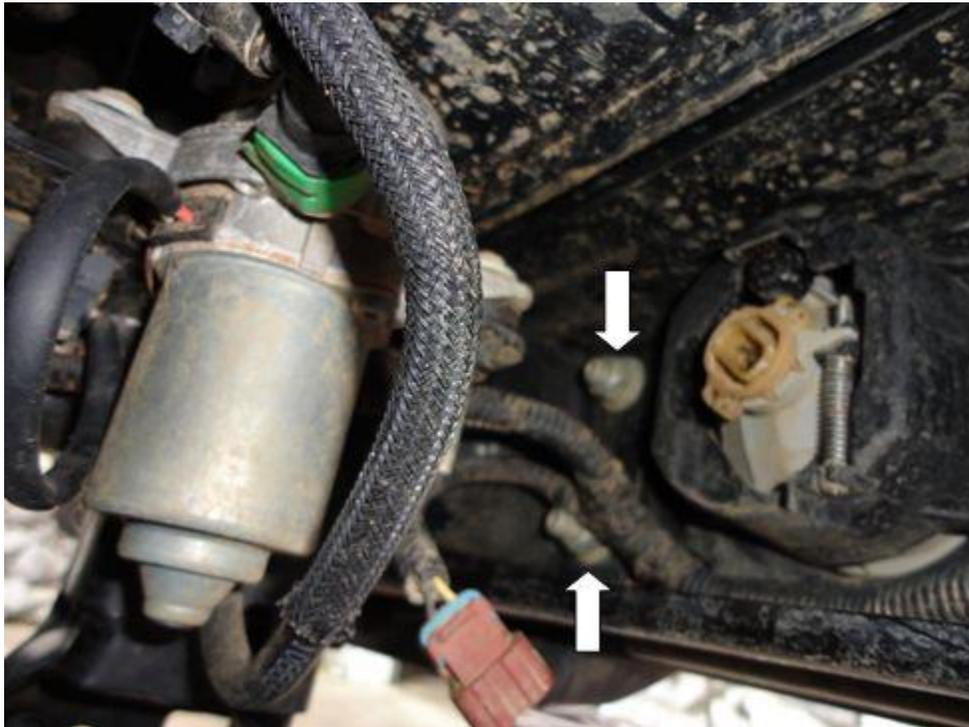
6. Set factory bumper bolts and backing plates aside. You will not need these to install the new bumper.
