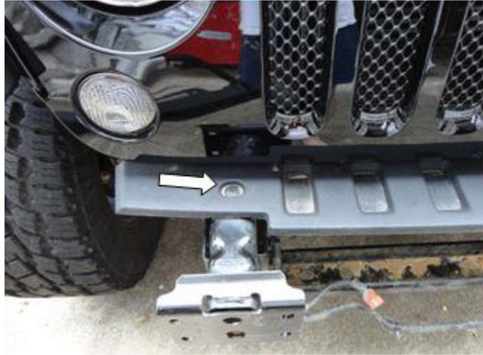
9. From inside the factory bumper, remove the factory fog lights by removing the 4 Phillips head screws. Repeat for other side.
