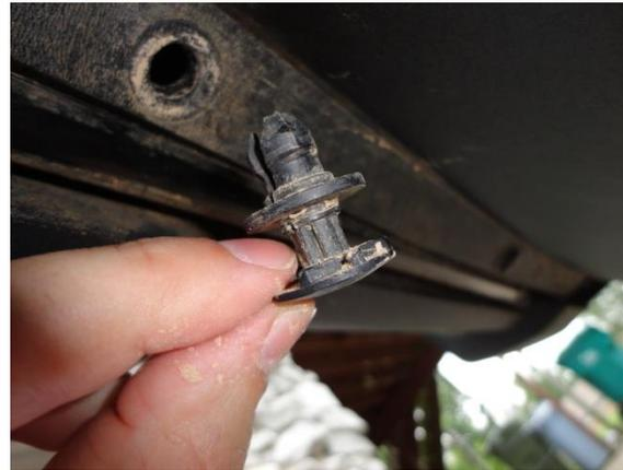
2. After removing the four plastic plugs, the air dam will swing down. Remove the two additional plastic plugs inside the air dam on the hinges.
