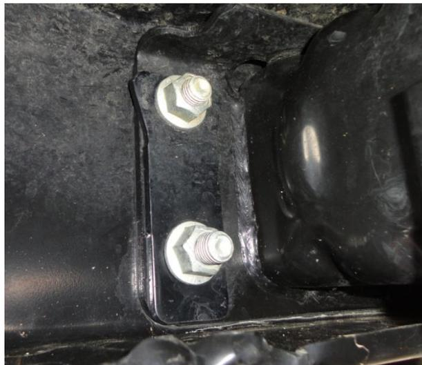
5. The driver's side inner bumper bolts may be hard to reach because the fuel pump is mounted nearby. Use a deep-well 18 mm socket, swivel and ratchet to remove these two bumper bolts.
