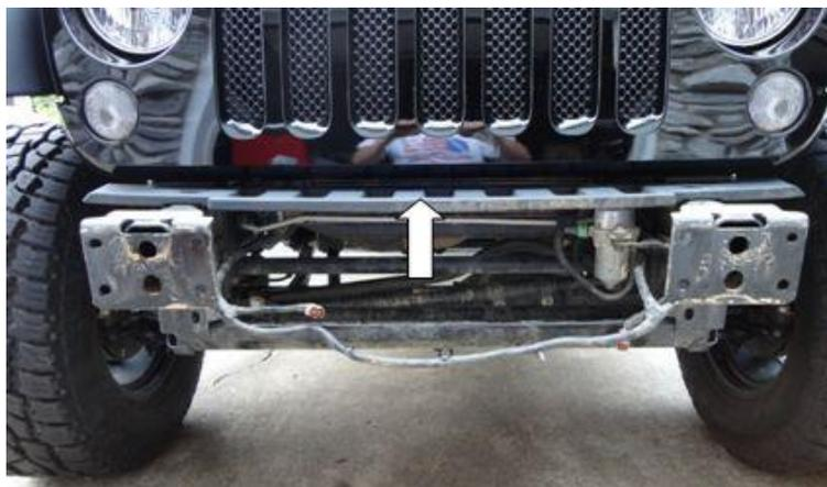
8. *Optional:* You *may* remove the bumper splash guard at this time but it is not necessary to fit the new bumper. To remove the splash guard, remove the two plastic Phillips head plugs on each side of the splash guard. Turn very gently as these are easy to strip out. If you strip out the Phillips head plugs, you can still remove the splash guard by prying underneath with a flat screwdriver.
