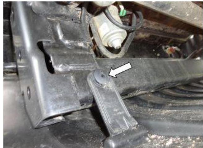
3. Remove the factory fog light connections by pushing the tab in on the brown connector and gently pulling out.
