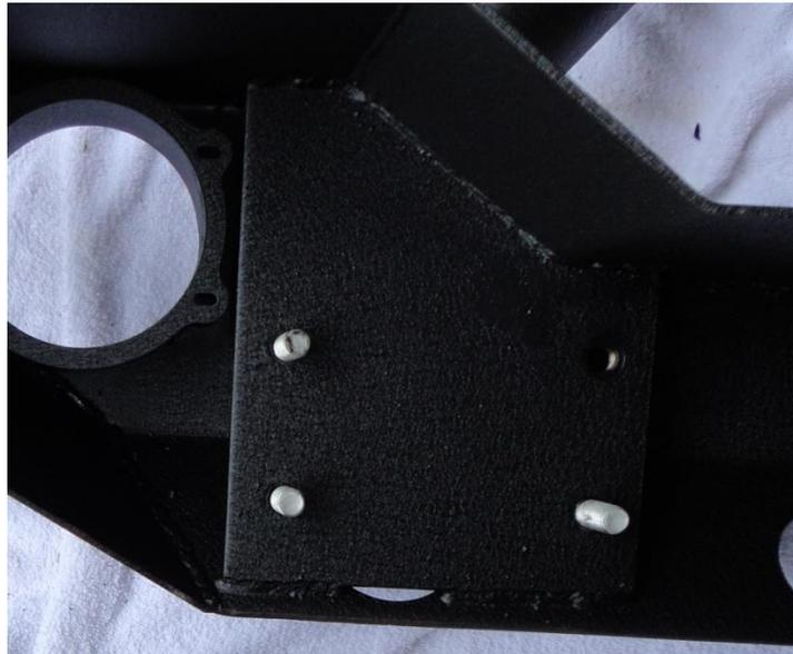
19. Torque the bumper mounting nuts/bolts to 75 foot-pounds.
