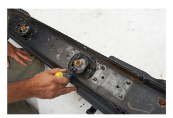
**STEP 4 //** To remove the fog lights, loosen the 4 phillips screws on each light.
