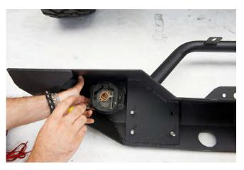
**STEP 5** // Reinstall the fog lights onto the new bumper by using the supplied bolt and screws to secure it into the housings.
