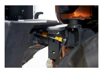
**STEP 2 //** Next, unplug the factory fog lights and loosen the (8) 19mm nuts holding the front bumper to the support beam of the vehicle.
