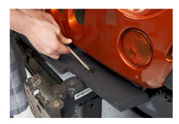
**STEP 3** // Remove the 2 push pins holding the top cover onto the vehicle
