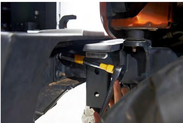
**STEP 2** // Next, unplug the factory fog lights and loosen the (8) 19mm nuts holding the front bumper to the support beam of the vehicle.
