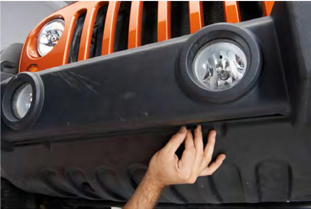
**STEP 1** // Remove the 6 pins holding the splash guard onto the vehicle
