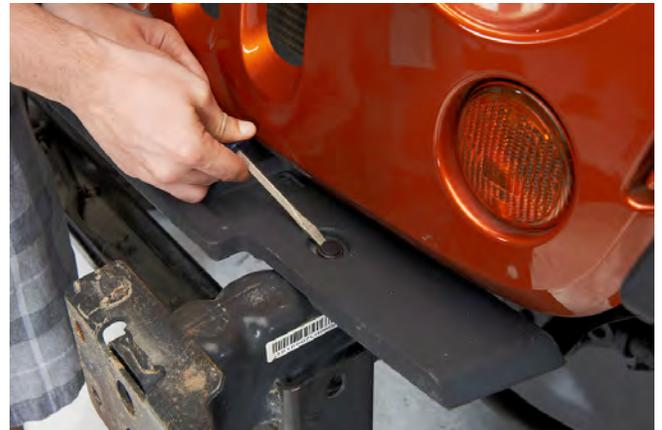
**STEP 3** // Remove the 2 push pins holding the top cover onto the vehicle
