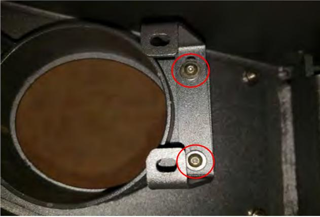
**STEP 5 //** Install the supplied bracket to the barricade bumper and then install the fog lights onto the bracket and bumper by using the supplied M4 hardware.
