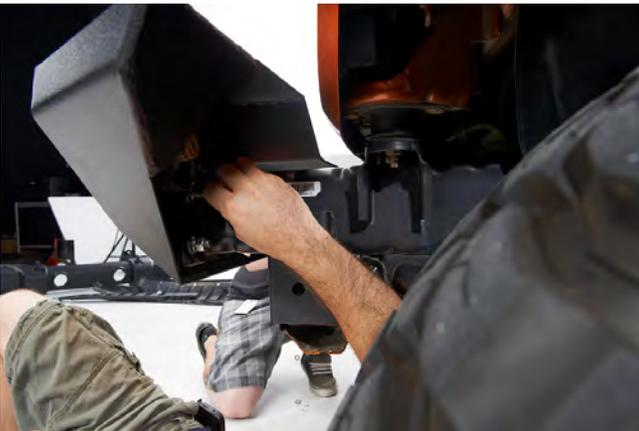
**STEP 6 //** Slide the bumper in place. Using the supplied washers and nuts, secure the bumper to the frame.
