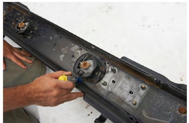
**STEP 4** // To remove the fog lights, loosen the 4 phillips screws on each light.
