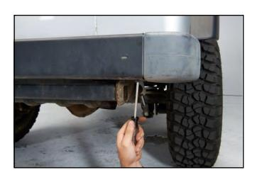
**STEP 2** // Remove the Torx screws, on the top and bottom, holding the end caps on the rear bumper and remove them.
