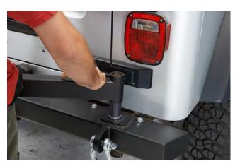
**STEP 10 //** Install the swing arm by sliding it over the post on the bumper. \*Note it may help to grease the post for smoother operation.
