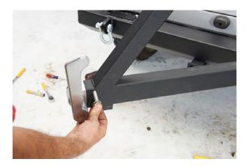
**STEP 12** // Slide the latch assembly into the swing arm and secure using the 17mm bolts and nuts.
