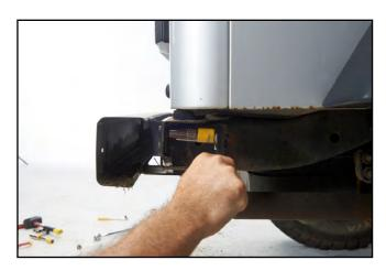
**STEP 3** // Using an 18mm socket, remove the (4) bolts securing the rear bumper.
