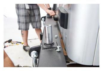
**STEP 8 //** Using the 18mm supplied bolts, washers and nuts, install the rear bumper onto the vehicle, leaving it loose for adjustment.
