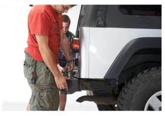
**STEP 6** // Slide the new bumper into position on the mounting brackets and line the 4 holes on the top of the bumper up with the 4 holes on the mounting plates.
