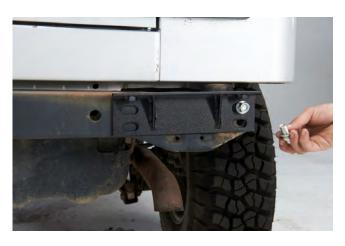
**STEP 5** // Using the supplied brackets and 18mm hardware, mount them to the vehicle in the factory mounting holes as pictured.
