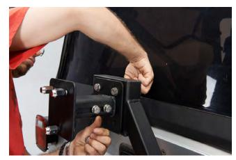
**STEP 13** // Finally, install the rear tire carrier onto the rear swing arm using the (4) 18mm bolts and nuts and tighten them down. Then, reinstall the rear tire.
