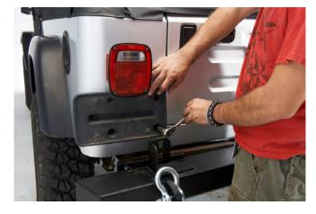
**STEP 7** // You may have to remove the plate bracket for extra clearance. Using a 10mm socket, remove the plate holder.
