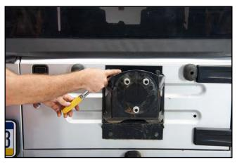
**STEP 1 //** Remove the rear tire and the (4) 13mm bolts securing the tire carrier.
