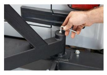
**STEP 11** // Install the top cap and secure it using the hex bolt.
